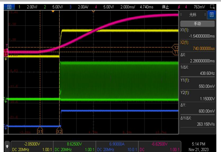
Fig 8 Enable Start up ( V_{in}=12V , V_{out}=3.3V , I_{LOAD}=2A )
