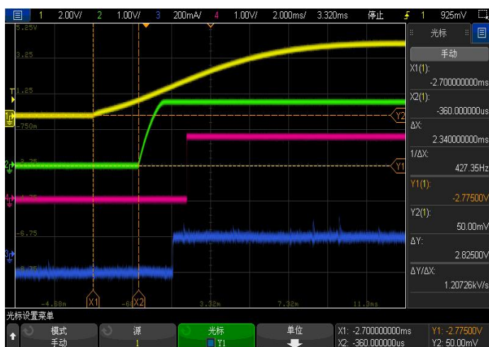
Fig 3. EN Power ON, I_{OUT}=200mA
