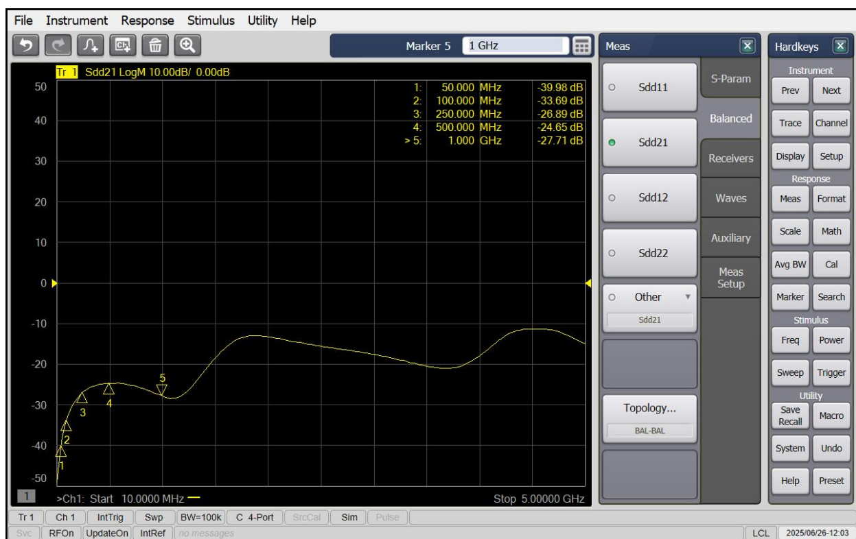
Fig 9. Switch Off Isolation
